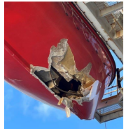
Figure 1: Lifeboat damage sustained from ruptured compressed air cylinder.
