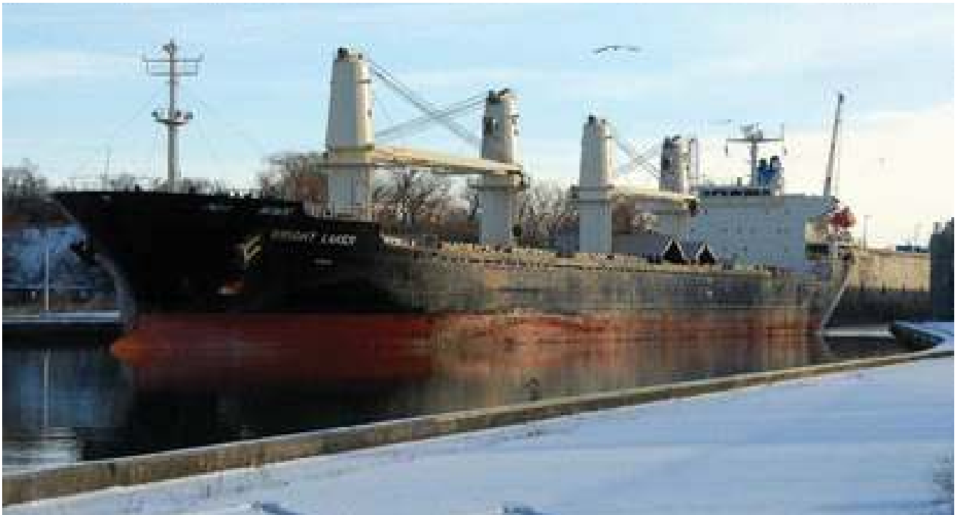
Ocean freighter transiting St. Lawrence Seaway: 1 inch reduction in water level means 100 tons less cargo.
