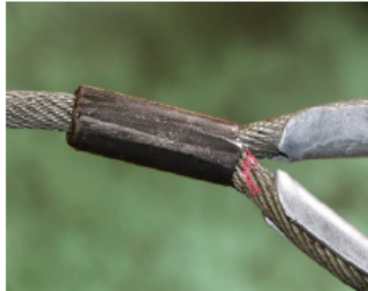
Figure 3: Fitting is deformed with "ridges" of extra material present from over-crimping.
