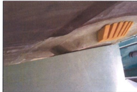
Lead portion of the stabilizer systems mounting and backing looking aft and outboard.
